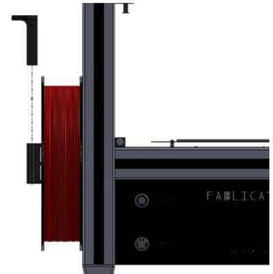
8. Loop the filament over the extrusion, and into the entrance of the extruder (marked with a yellow arrow)
