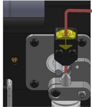
7. If the filament starts to push down into the nozzle continue until the clog has passed and is re-melted in the nozzle tip.
