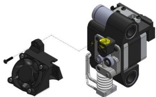
17. After double checking the Driver set screw, idler screw, and fan shroud screws are all snug, the extruder is ready to be used again.
