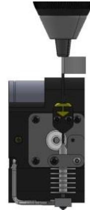
Once the filament path is all clear, heat up the nozzle in the Fablicator interface and manually push filament down into the nozzle before doing any
