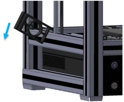
Attach the clear magnetic panels to the machine.
