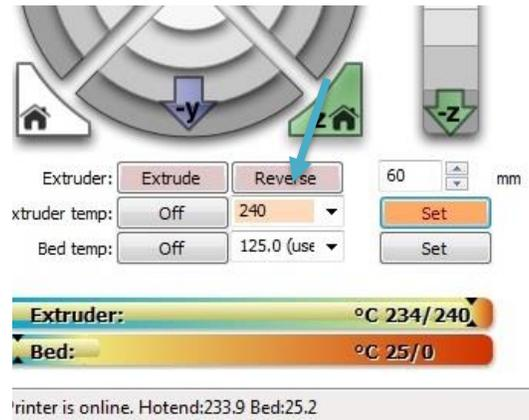
6. After the extruder motor stops, lightly pull on the filament and it should come out of the extruder assembly.
